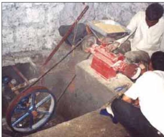
(e) Improved micro hydro site for electricity generation and rice milling in Uttarakhand, India.
