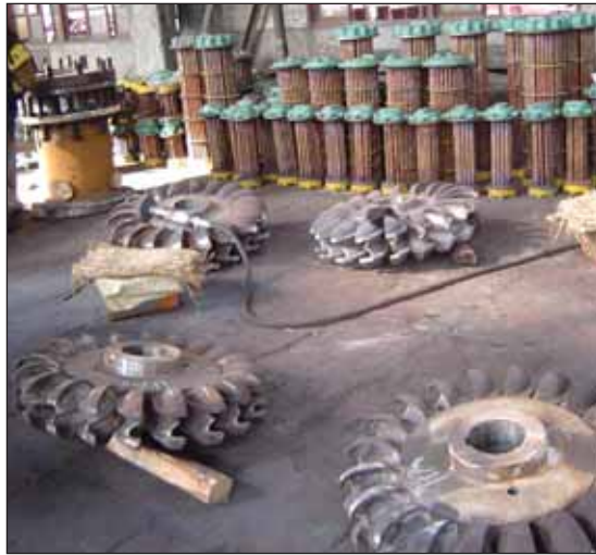
(c) Mass production of Chinese Pelton turbines.
