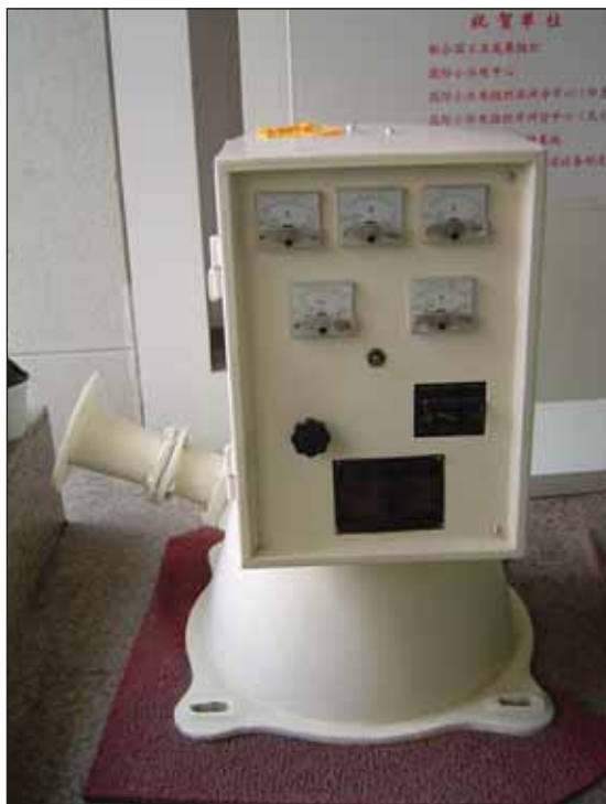
(g) A 7.5 kW micro hydro packaged system made by the Zheng He Water Turbine Factory, Fujian Province, China.
